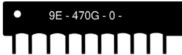
FIGURE 7.3 The SIL resistor pictured here has nine resistors, each delivering 47Ω. The code reads 470, which equals 47 \times 10^0 , or 47.
