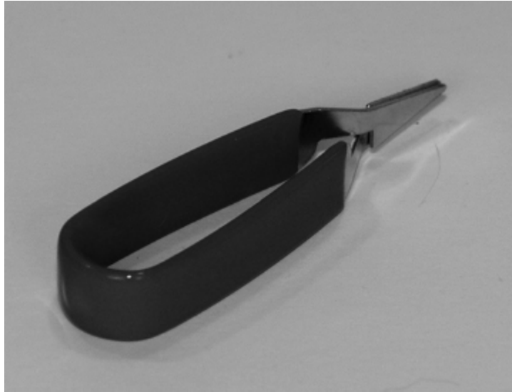
FIGURE 4.11 A heat sink with an insulated handle.
