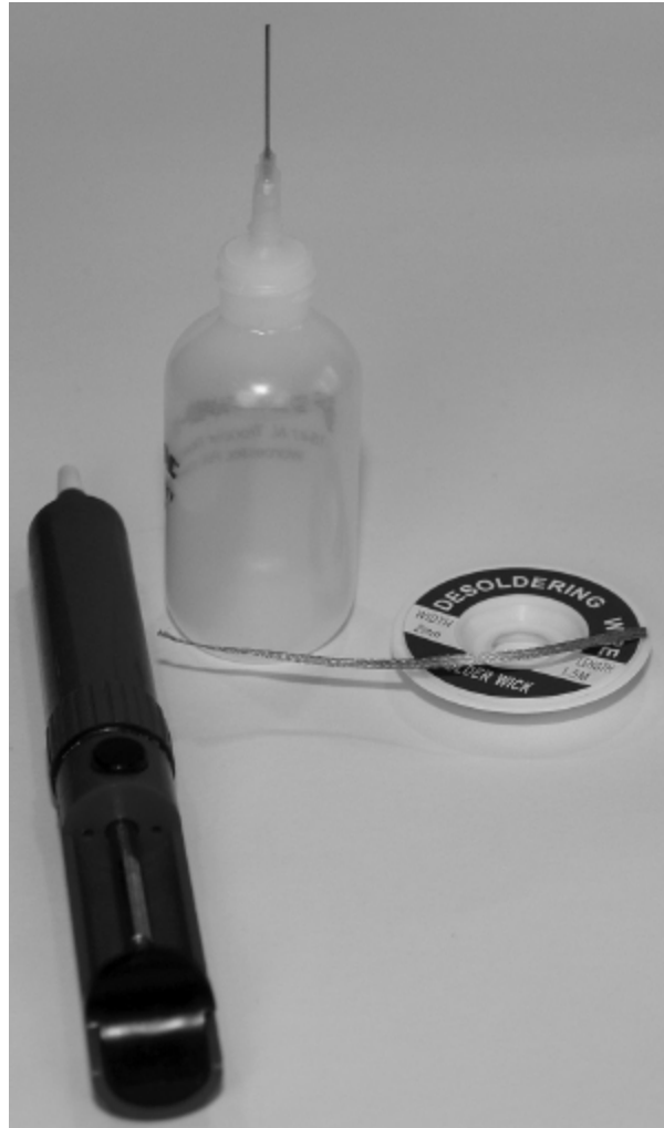
FIGURE 4.10 From left to right, a solder sucker, flux bottle, and solder wick.
