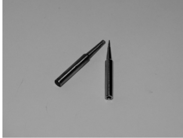
FIGURE 12.5 You'll want a flat-head tip (left) and a fine-point tip (right) for your soldering iron.
