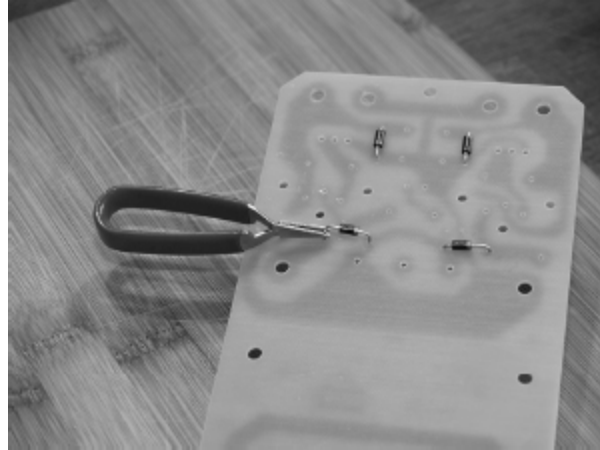
FIGURE 12.6 Using a heat sink.
